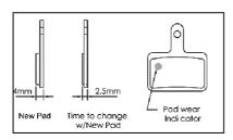
Fig. I-1 Identify worn brake pads
