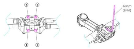
Fig. E-1 Torqueing sequence
