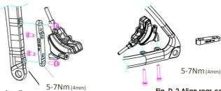
Fig. D-1 Align front-caliper with fork mounting holes.
